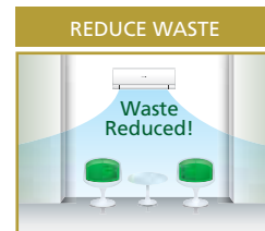
Gradually reduces cooling power by an amount equivalent to increasing the set temperature by 2 degrees Celsius.
