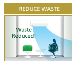
Reduces cooling the unoccupied area of the room.
