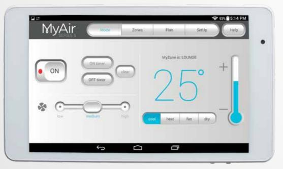
The home screen gives you an overview of the air-conditioning status. Adjust the central temperature from this screen, or tap through to zones to fine-tune the airflow to every room
